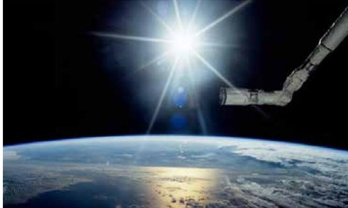
*Image of the Canadarm wrist joint and forearm covered with insulation to protect components from the heat generated by the sun's radiation. (Credit NASA)*
