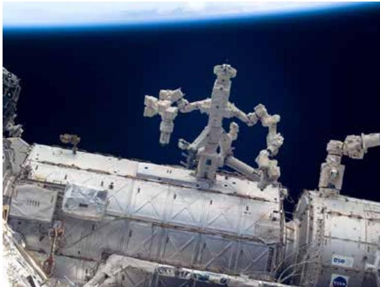
*Dextre* is seen in this image performing installation work on the payload *Destiny*. Note *Canadarm2* attached to an End Effector to the right. (Credit NASA)
