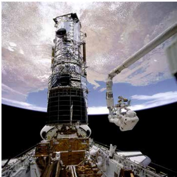
*To repair the HST it was temporarily stowed in a pallet at the rear of the orbiter. Note astronaut being moved by the Canadarm to effect repairs. The HST has a high orbit hence the earth's curvature is seen more clearly. (Credit NASA)*
