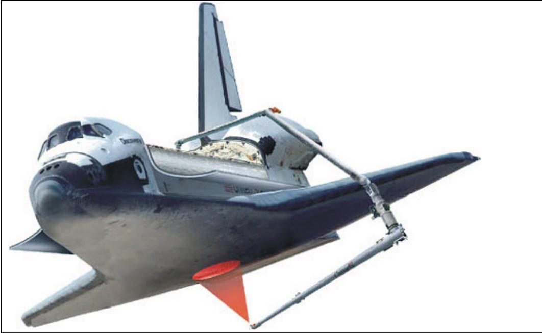
***A schematic showing how the boom assembly and Neptec Laser Camera System (in red) could be employed to inspect the heat shield tiles located on the underside of the Orbiter's wing. (Credit NASA)***
