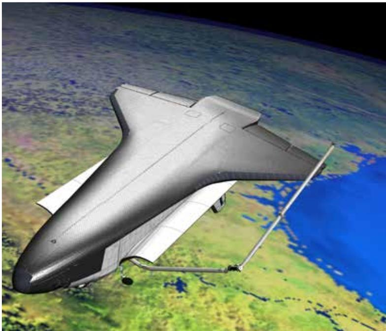
***Schematic showing how the Orbiter exposed its underside to the International Space Station cameras, which were analyzed to confirm no damage had occurred to the tiles on lift-off. (Credit NASA)***
