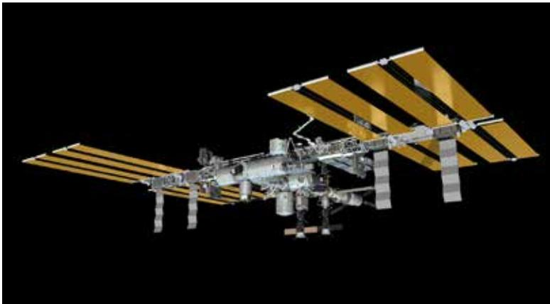
*A schematic showing the truss structure which spans the entire space station including the massive solar arrays for powering the ISS. (Credit NASA)*
