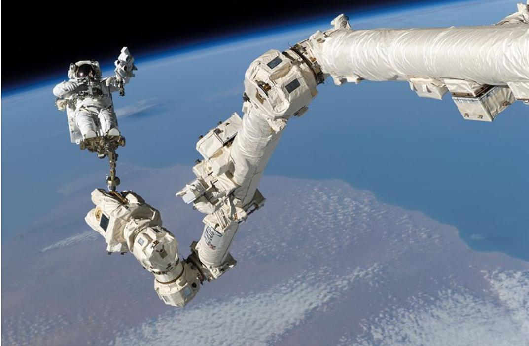
***A photograph of Canadarm2 with an astronaut firmly held by foot restraints. Canadarm2 worked in harmony with the Canadian designed Dextre and the American Mobile Base System to attach and service modules to the ISS. (Credit NASA)***
