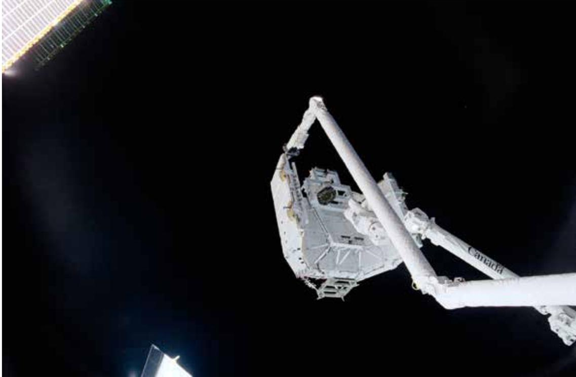
*An image showing the "Canadarm Handshake". In this photograph the ISS based Canadarm2 is transferring the pallet on which it was transported to the ISS back to the Shuttle's Canadarm for its return journey to earth. (Credit NASA)*
