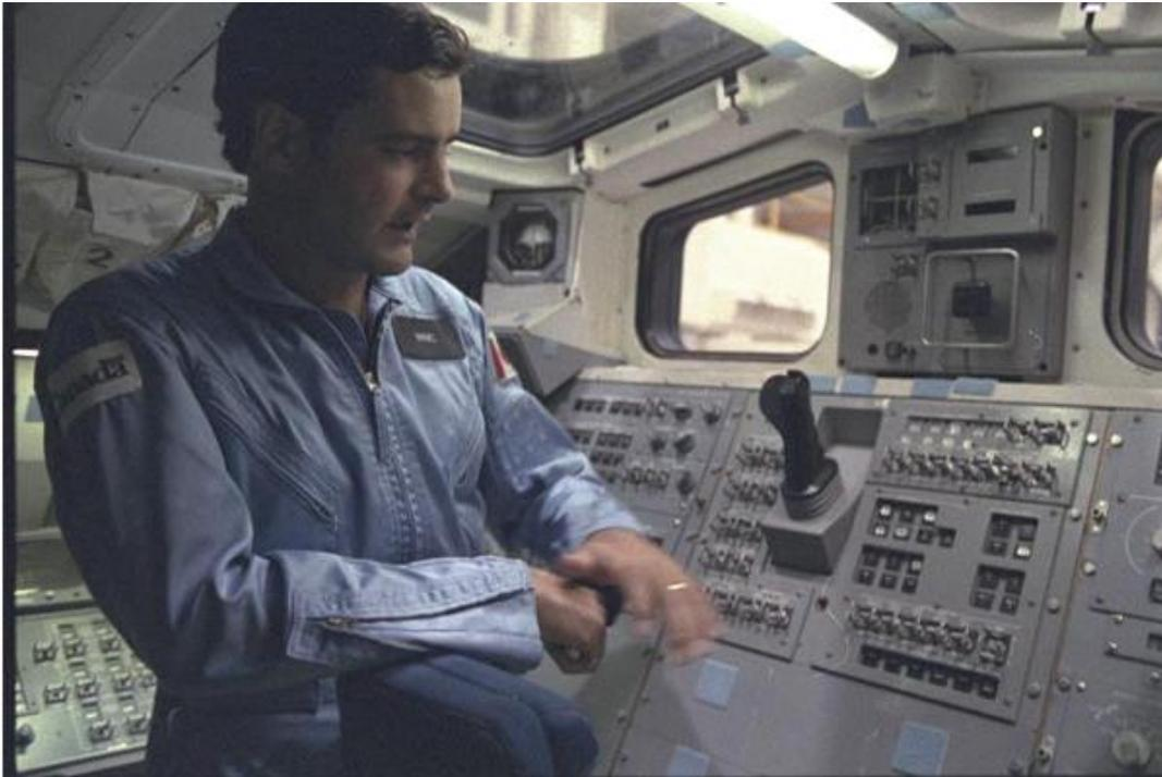
***Canadian Mission Specialist Mark Garneau beside the Canadarm control console. The arm's rotational controller is the larger device adjacent to his left hand. The translation controller is above and slightly to the right in the square fitting. (Credit NASA)***
