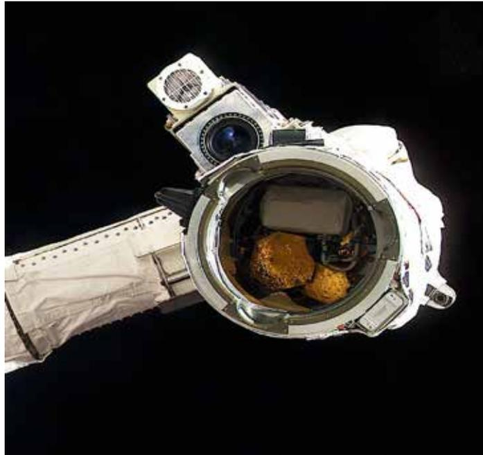
*Photograph of the Neptec Laser and Camera System mounted on top of the Orbiter Boom Assembly (in turn mounted on the end of the Canadarm). (Credit NASA)*
