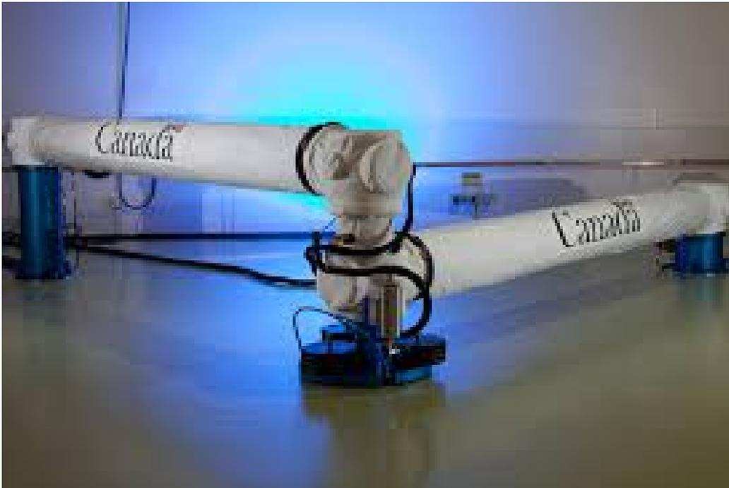
*A Canadarm being tested on the ground for space flight. It is supported by air bearings to simulate operation in the weightlessness of space. On earth, it cannot support its own weight. (Credit DSMA Atcon Ltd.)*
