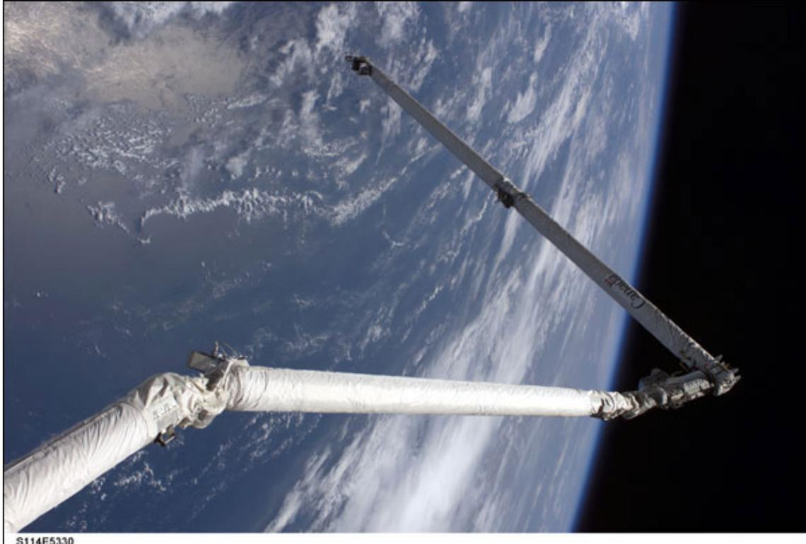
**A photo of the boom attachments, which extend the length of the Canadarm. The Neptec LCS is mounted on the end of the OBSS and allows the astronauts to inspect the tiles for damage while on-orbit. These critical heat shield tiles are located on the leading edge and underside of the Orbiter's wing. (Credit NASA)**
