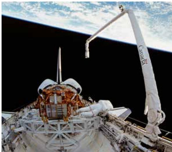
**Photo looking rearward from the Shuttle's cabin shows the *Canadarm* mounted on the port side of the cargo bay. (Credit MDA)**
