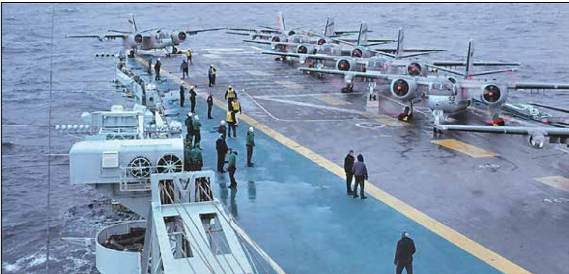
*In very much less than ideal weather conditions, a mass runup of all the VS 880 and single VX 10 (at rear) Trackers on deck is seen preparatory to the Carquals and capabilities being performed. (Seth Grossmith Photo)*
