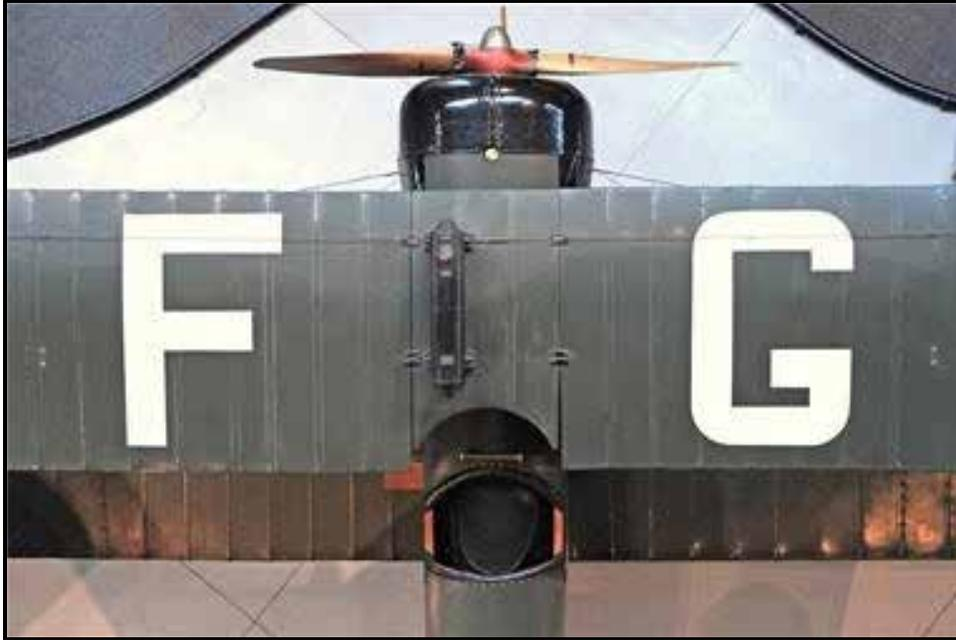
*Overhead shot of G-CYFG showing original fuel tank location of on upper wing centre section. This tank was removed on G-CYCK and G-CYEI and replaced by an internal tank to facilitate safer disassembly and transportation during the 1967 flying display season (Bill Upton photo).*
