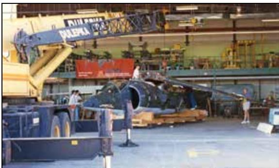
*The skilled staff of the NAM gently lowers the complete wing assembly onto the fuselage of 158966 in July 1997. Such a technique permits complete access to the engine for ease of removal or maintenance as necessary. (CAvM Photo 35-66-22)*
