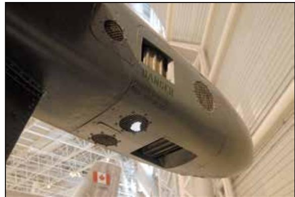
*Tailcone RCV pitch and yaw (each side) control nozzles. (Bill Upton Photo)*
