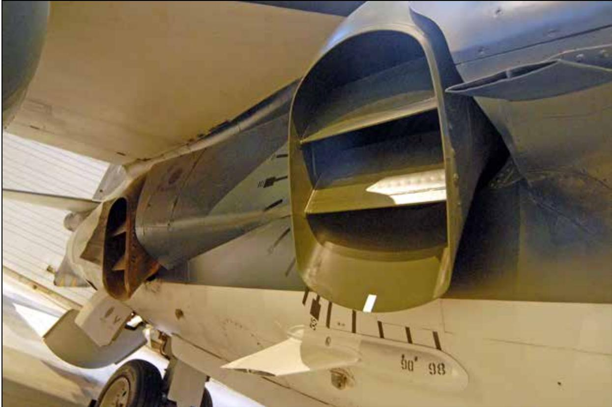
*An angle of rotation index reference marking is seen on the forward (cool) starboard engine exhaust nozzle. This would align with the fuselage's black angle indicator lines as the pilot selects a required thrust vector angle thus rotating the nozzles in symmetry. Seemingly impossible rearward transitions of the aircraft during level flight are possible when all of the exhaust nozzles are rotated forward on the Throttle Box by the pilot to the 98-degree markings. (Bill Upton Photo)*
