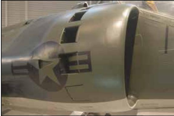
*Around the exterior of each intake are a series of fully floating supplementary suction intake doors. A ram air scoop for engine cooling is seen within the 'star' of the national insignia. (Bill Upton Photo)*
