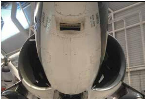
*Under the nose RCV pitch control nozzle installation. (Bill Upton Photo)*
