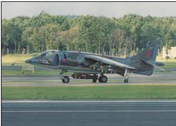
*A RAF Harrier GR.1A of 233 OCU is displayed loaded with BL755 Cluster Bomb Units hanging on all the wing stations. (Photo Courtesy BAe/Bill Upton Collection)*
