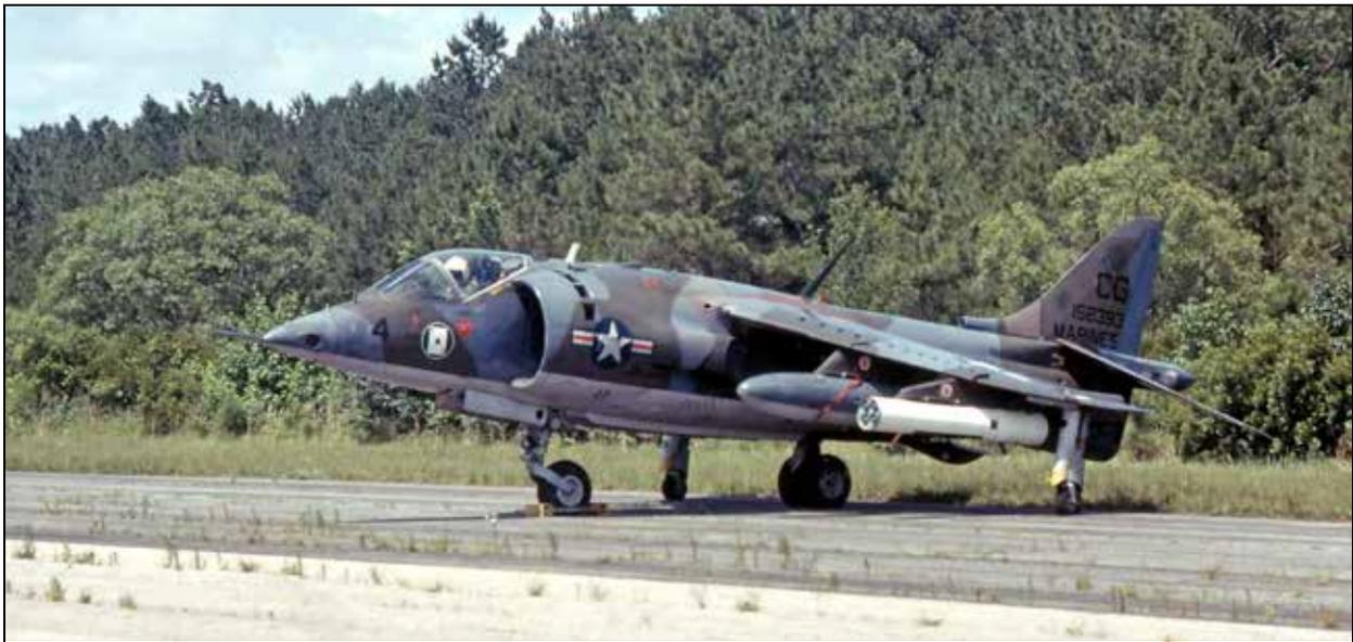
*The 10<sup>th</sup> production AV-8A Harrier 158393 (XW653) sporting underwing fuel tanks and Zuni rocket pods is seen at Marine Corps Air Station (MCAS) Cherry Point, North Carolina, in VMA-231 (CG-4) markings during 1974. (Bill Upton Collection)*
