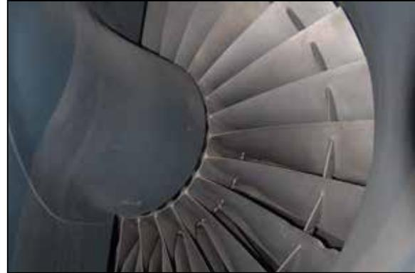
*The compressor fan face of the Pegasus 103 turbofan engine is readily visible in the bulbous port side air intake. The large intake centerbody fairing supports the front part of the engine. (Bill Upton Photo)*
