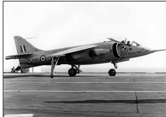
*The prototype P.1127, XP831, piloted by Bill Bedford, performs the first ever jet V/STOL at-sea trials aboard HMS Ark Royal (R09) during February 1963. Round, segmented black and white targets, for photo calibration and tracking purposes, are clearly seen on the intake splitter and aft fuselage. A long instrumentation boom is attached at the nose of the aircraft. (Photo Courtesy BAe/Bill Upton Collection)*
