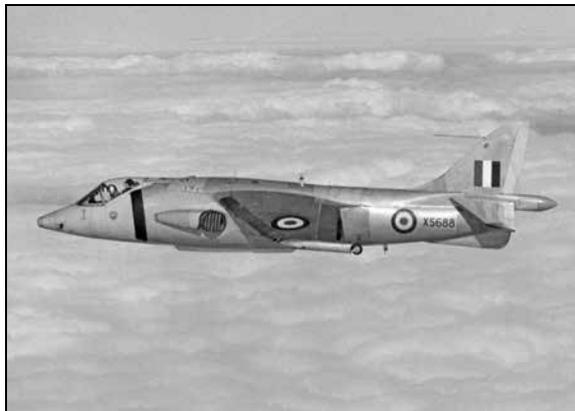
*The first Kestrel F(GA) Mk.1, XS688, is seen on an early test flight in early 1964 bearing the standard RAF roundels and fin flash. Note the somewhat longer and more humpbacked appearance of the fuselage compared to the original P.1127 prototype. A long nose mounted instrumentation boom was originally installed for test purposes, then soon dispensed with, on this first of nine aircraft and was replaced by a nose mounted combat strike camera. (Photo Courtesy BAe/Bill Upton Collection)*
