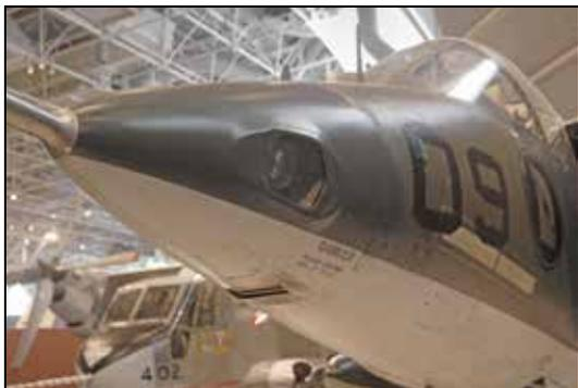
*The F95 oblique combat camera and its view port installation are still on 158966. A small, swiveling weathervane (missing here) is normally installed atop the small post directly ahead of the cockpit. This is used as a reference for the pilot to hold the Harrier's nose into the wind during hovering flight. (Bill Upton Photo)*
