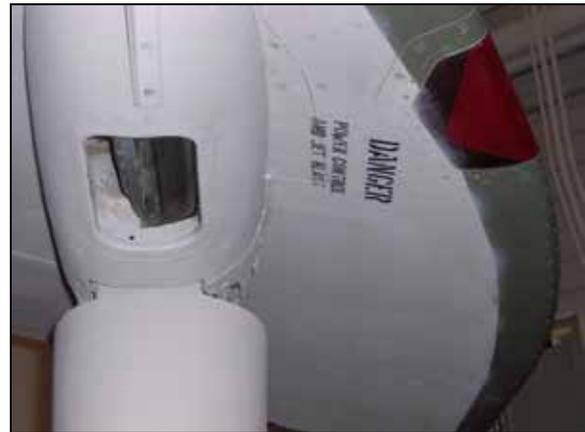
*Port lower wing RCV roll control nozzle. (Bill Upton Photo)*
