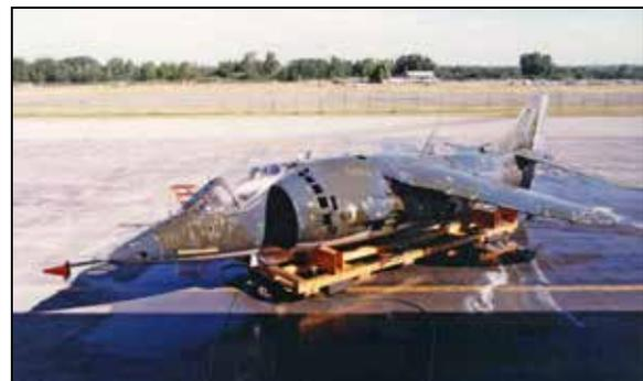
*By 3 September 1997, aircraft 158966 was nearing completion, with the wings and empennage mated, and was just about ready for some paintshop work. Remnants of the original squadron markings are still visible. (CAvM Photo 32994)*
